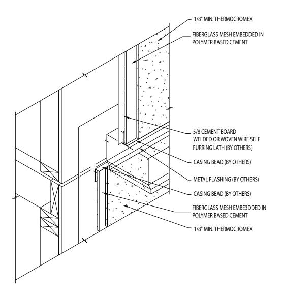
NOTE: All joints of cement board must be treated with 4" fiberglass mesh embedded in polymer based cement.
